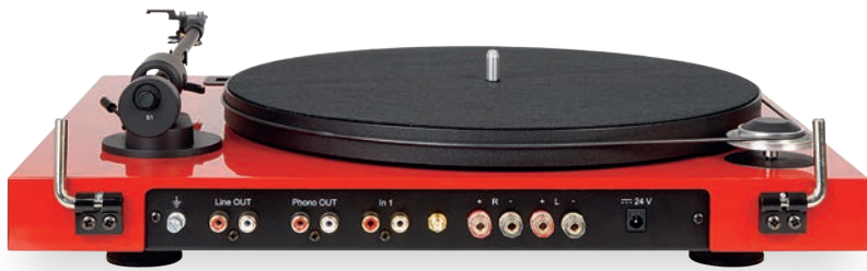
ABOVE: No ordinary turntable! RCA sockets are provided for a native (tonearm) output, an RIAA-equalised output and a line input. A Bluetooth antenna connection sits alongside 4mm terminals/binding posts for speaker cables. Power is via a 24V PSU
